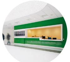
The reception is a good example of how to solve a physical barrier using universal design. The counter is simply designed in two different levels, which means that anyone can get information and help in an equal manner and at eye-level, whether they are standing or sitting in a wheelchair.
